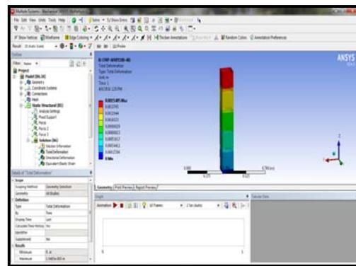
**Fig. 8: Deflection for CFRP-AFRP (100-40) column**
