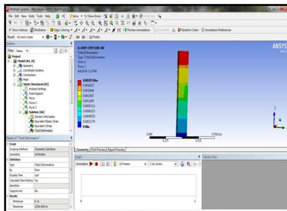
**Fig. 9: Deflection for AFRP-CFRP (100-40)**
