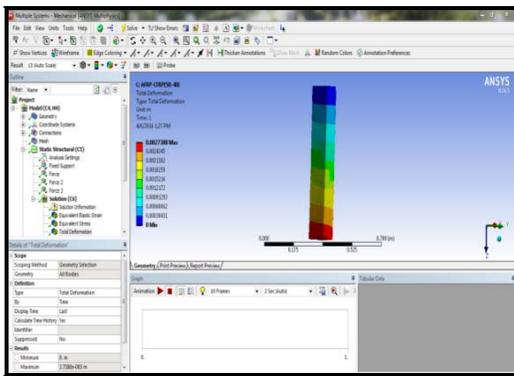
**Fig. 7: Deflection for AFRP-CFRP (50-40) column**
