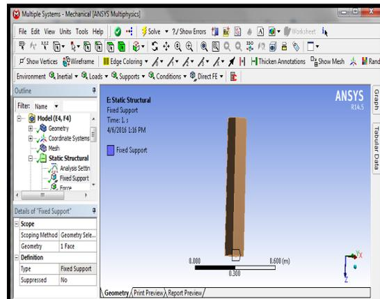
**Fig. 1(B): Applying support conditions for SHS**
