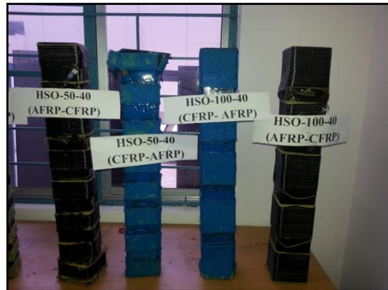
Fig. 4: Modes of failure
