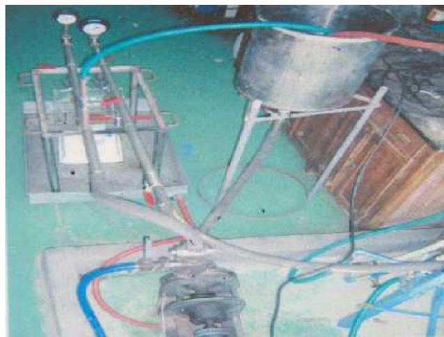
Figure 2 : Diagrams of experimental setup shows the cross flow membrane module installed in setup
