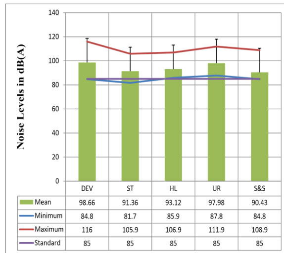
FIG. 8. Noise exposure levels of activity areas in the Kwasi Mensah Shaft.
