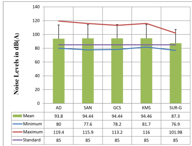
FIG. 1. Mine wide operational shafts personal noise exposure profile.
