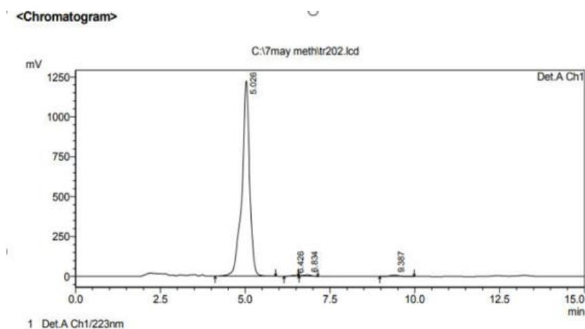
FIG.2. The HPLC chromatogram of Andrographolide reference standard (BNPL/RFSTD/002).
