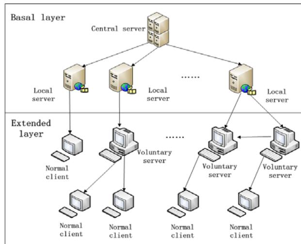
Figure 2 : The video grid of scalable architecture
