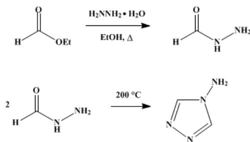
FIG. 5. Synthesis of 1,2,4-Triazoles
