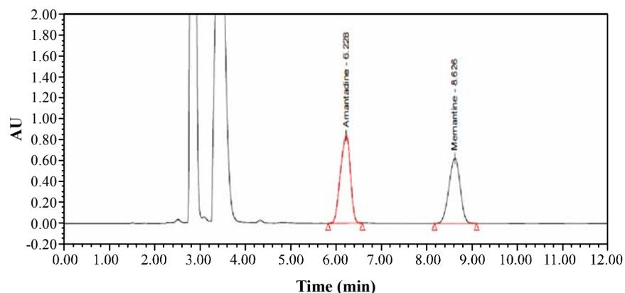
Fig. 5: Standard chromatograms of amantadine hydrochloride
