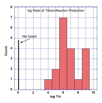
FIG. 1. Histogram of independent studies that measured both tritium and neutron emission [32], with COUNT giving the number of times the noted log T/n value was reported. The clustering of values suggests a relationship exists between tritium and neutron production, but not the same one known to result from hot fusion.
