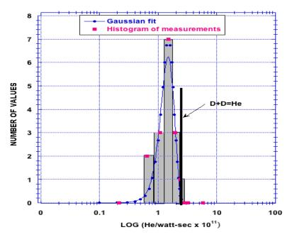
FIG. 2. Summary of 17 measurements of both helium and energy production during the same study [32]. Superimposed on the distribution of values is a fit to the Gaussian error function. The fit is typical of an expected amount of random error being present in the measurements. The value for this ratio resulting from deuterium-deuterium (d-d) fusion is known to be 23.8 MeV for each nucleus of helium made.
