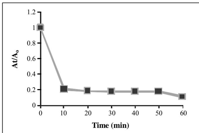
**Fig. 4: The remaining percentage of adsorption BBG over the catalyst**
