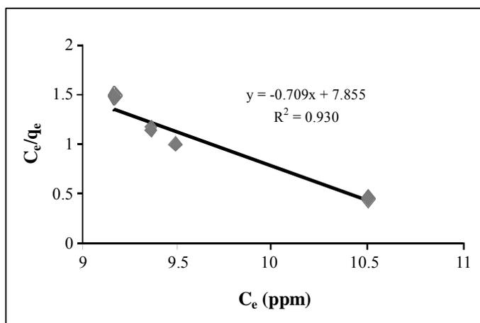
**Fig. 5: Langmuir adsorption isotherm for adsorption of BBG on the prepared catalyst**
