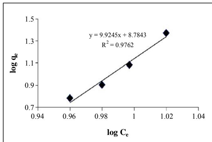
**Fig. 6: Freundlich adsorption isotherm for adsorption of BBG over the catalyst**
