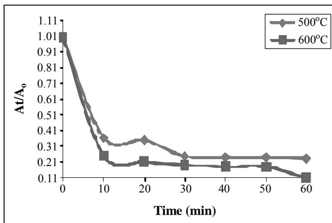
**Fig. 3: Removal of BBG over prepared catalyst under calcination at different temperatures 500, 600°C**
