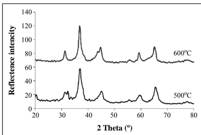
**Fig. 2: X-ray patterns for the prepared catalyst after calcination at different temperatures 500 and 600°C**
