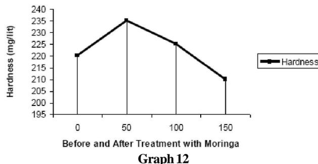
In general, the softening mechanism was postulated to be a combination of adsorption and precipitation of the soluble hardness causing ions to insoluble solids / flocs<sup>[6]</sup>. By the above study, the desirable concentration of M.O. is 150mg/L is for Sample-1 and Sample-
