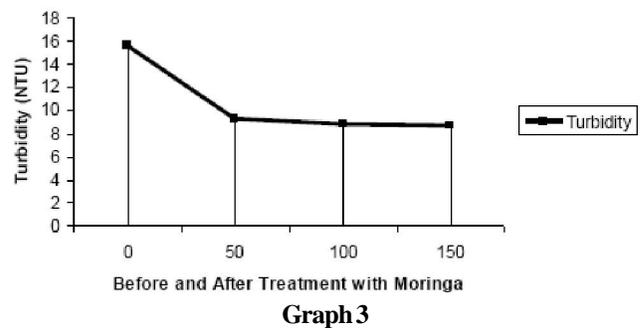
The above observation may be due to an improvement in the flock size and flock was settled rapidly. The overdosing resulted in the saturation of the polymer bridge sites and caused destabilization of the destabilized particles due to insufficient number of particles to form more inter-particle bridges. The high positive
