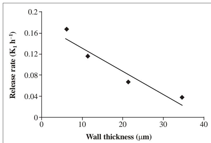
**Fig. 2: Relationship between wall thickness and release rate (K<sub>1</sub>) for starch acetate microcapsules of nifedipine**
