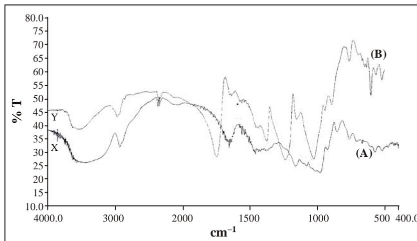
**Fig. 1: FTIR spectra of potato starch (A) and starch acetate (B)**
