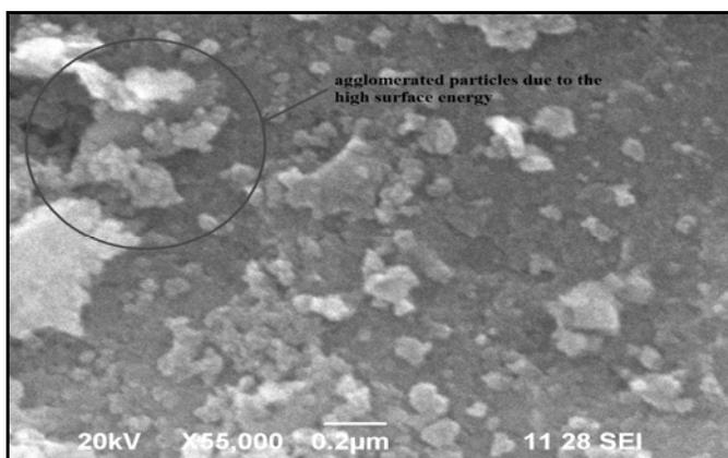
**Fig. 2:** SEM image of ZnS nanoparticles
