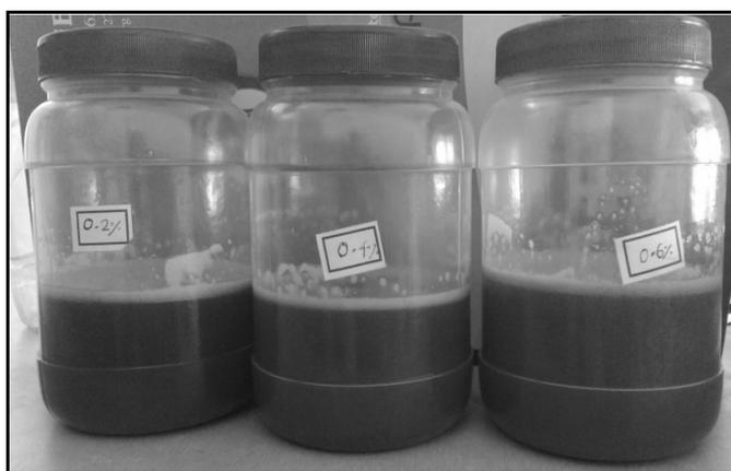
**Fig. 4: Ultrasonically prepared ZnS-gear lubricant oil nanofluids**
