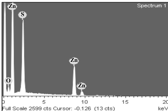
**Fig. 3:** EDS analysis of ZnS nanoparticles
