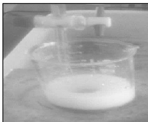
Step 2: Addition of sodium sulphide
