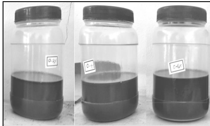
**Fig. 5: Photograph of different concentrations of nanofluids after 10 days**
