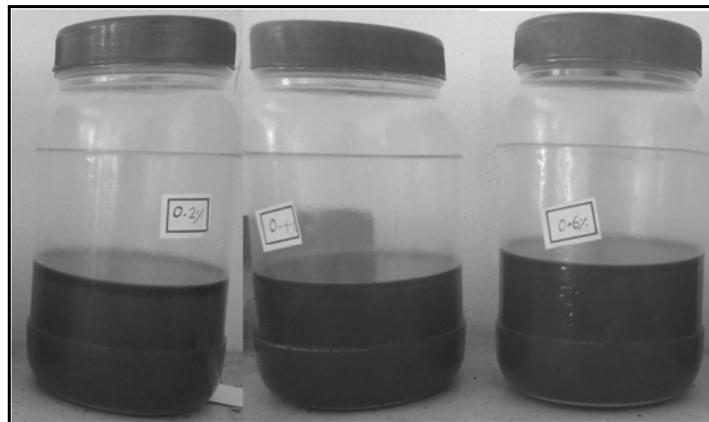
**Fig. 6: Photograph of different concentrations of nanofluids after 18 days**
