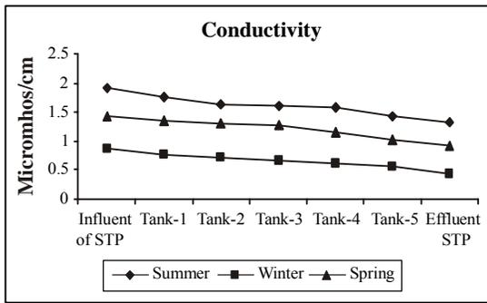
**Fig. 3: Seasonal variation of electrical conductivity in sewage treatment plant**
