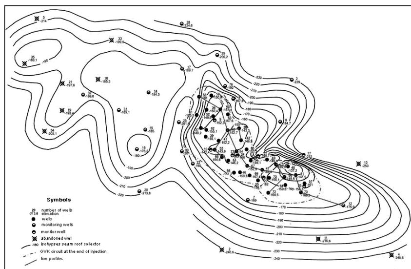
**Fig. 1: Contour map of “Akirtobe” UGS confining reservoir bed**
