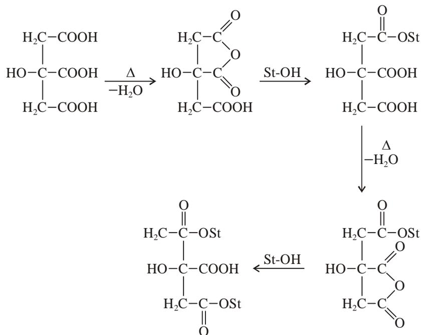
**Fig. 1: Starch–citric acid reaction**
