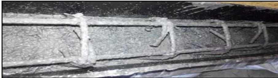
**Fig. 2: Casting of SIFCON beam**
