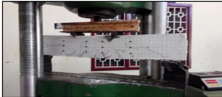
**Fig. 10: Crack pattern**
