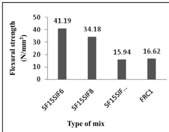
Fig. 4(b): Type of mix vs Flexural strength
