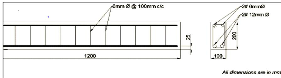
**Fig. 1: Beam reinforcement details**
