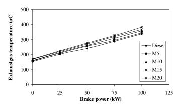
Fig. 5: Exhaustgas temperature Vs brake power
