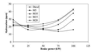
Fig. 7: Hydrocarbon emission Vs brake power
