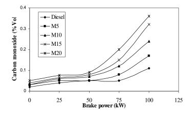
Fig. 6: Carbon monoxide emission Vs brake power
