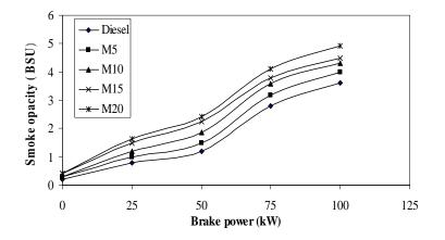
Fig. 9: Smoke opacity Vs brake power
