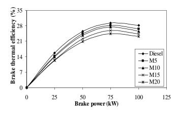
Fig. 3: Brake thermal efficiency Vs brake power
