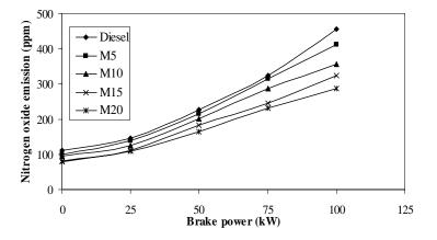
Fig. 8: Nitrogen oxide emission Vs brake power
