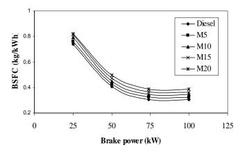
Fig. 4: Brake specific fuel consumption Vs Brake power
