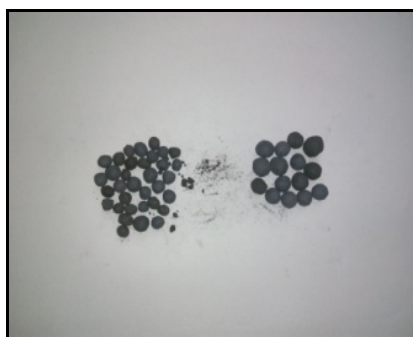
Fig. 6: Samples of 3 mm granules before and after coking and sample of different size of granules 3 mm and 6-10 mm
