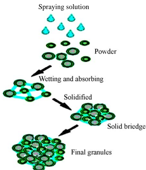
Fig. 1: Process principle of granulation
