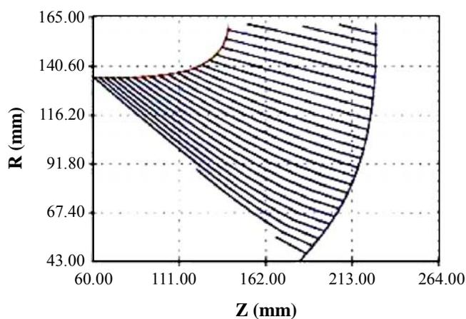
**Fig. 2: Impeller A blade cross-sections**
