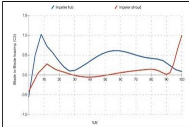
Fig. 7: Impeller A blade loading predicted from simplified Q3D procedure
