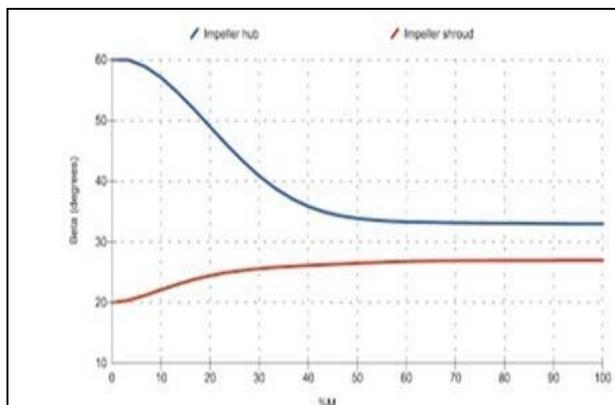
**Fig. 5: Blade angles distributions along hub and shroud for impeller A**
