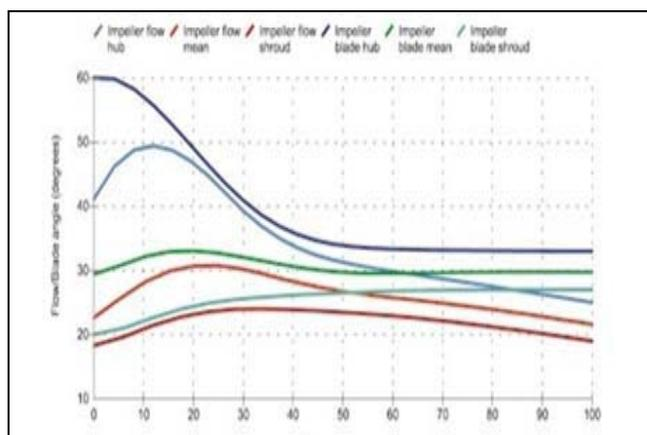
**Fig. 6: Flow and blade angles distributions along three blade**
