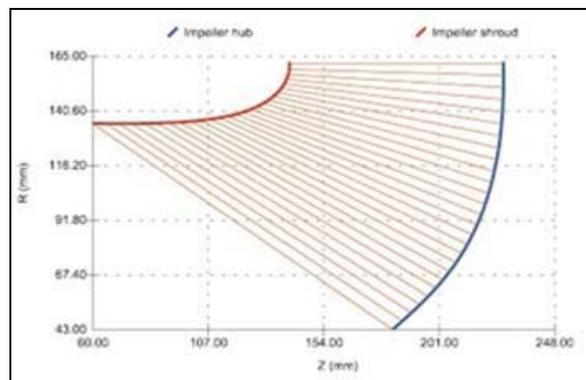
**Fig. 4: Meridional profile of impeller A with meshing for Q3D analysis**
