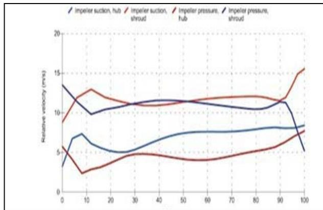
Fig. 8: Impeller A relative velocities distributions from simplified Q3D
