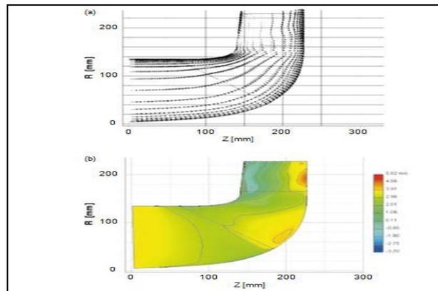
Fig. 9: Impeller A meridional velocity vectors at mid-passage
