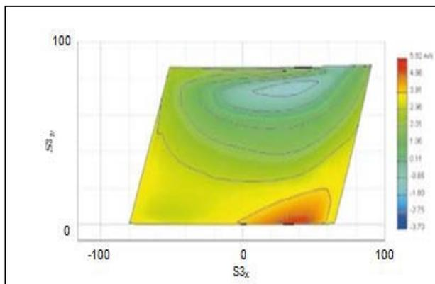
**Fig. 10: Impeller A meridional velocity distribution and velocity distribution at mid-passage immediately after TE**
