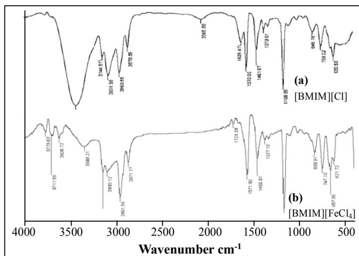
Fig. 1: FTIR Spectra of (a) ionic liquids [BMIM][Cl] and (b) modified ionic liquids [BMIM][FeCl<sub>4</sub>] based ionic liquids
