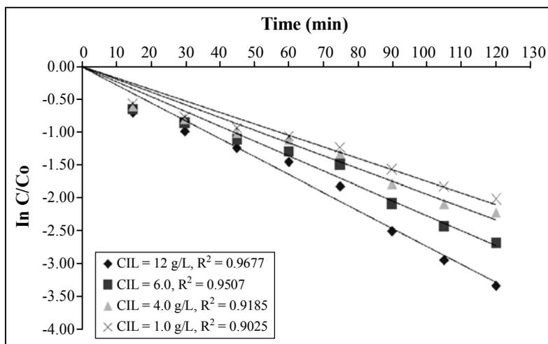
**Fig. 6: Effects of concentration of IL of mixed solution on the rate of TNT reduction**
