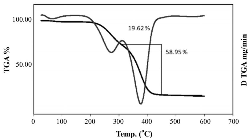
Fig. 2: DTGA & TGA results of  $[\text{BMIM}]\text{FeCl}_4$  based ionic liquid
