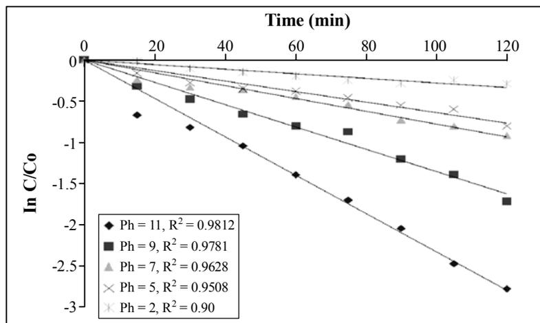
**Fig. 8: Effects of pH value of mixed solution on the rate of TNT reduction**
