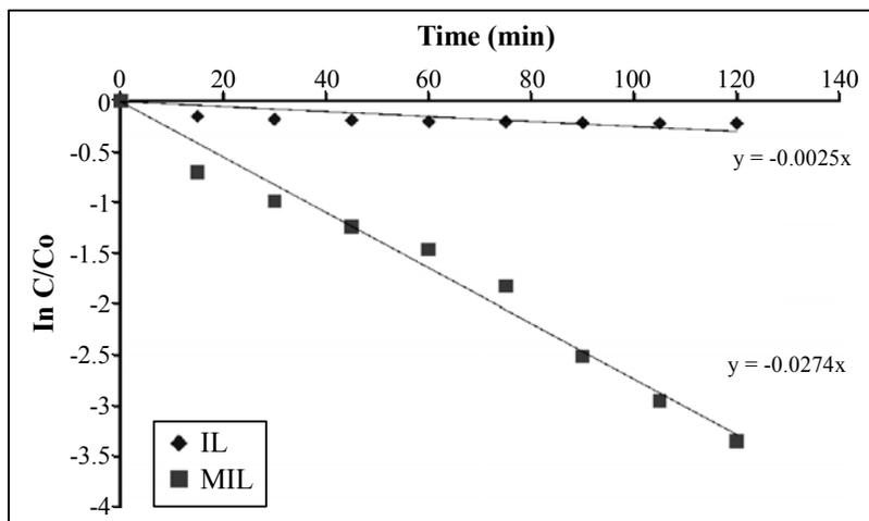
**Fig. 4: Relationship between logarithmic plots of TNT concentration versus time**
