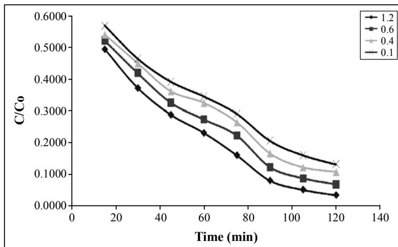
**Fig. 5: Residual TNT concentration with effect of MIL concentration**
