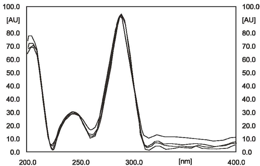
**Fig. 1: Densitogram obtained from pure protopine**
