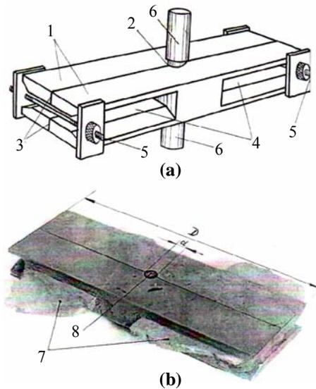
**Fig. 2: Device for testing a tensile strain of large twin rock specimens by coaxial punch method**
