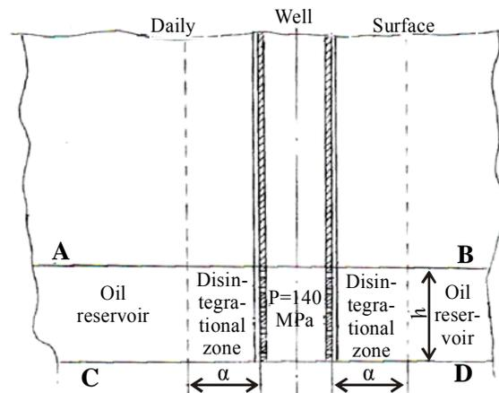
**Fig. 1: Oil reservoir and the well in the process of HF**
