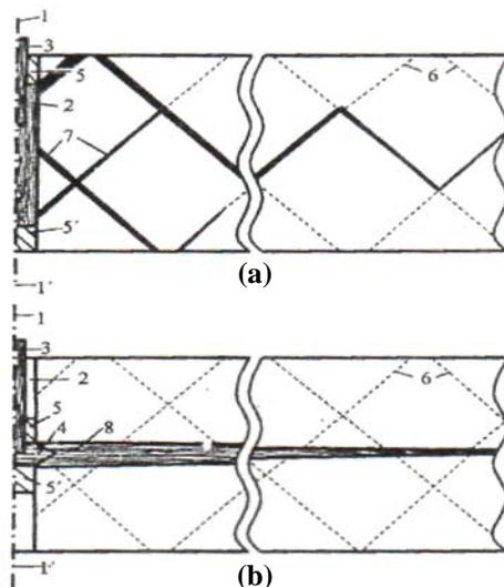
**Fig. 4: Scheme of fluid dismemberment (a) and oriented of fluid fracture (b) in the rock mass: 1-1'- a well axis; 2- a well; 3- a pipe for fluid pumping; 4- an initiating gap; 5-5'- upper and lower packers sealing well working space; 6- natural crack systems, 7-cracks of fluid dismemberment, 8- hydrofracturing cracks**
