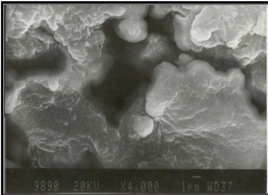
**Fig. 4: SEM photomicrograph of C.S of asymmetric membrane capsule (4000X magnification)**
