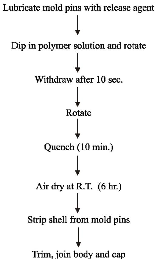
**Fig. 1: Manufacture of asymmetric membrane capsules by wet process method**
