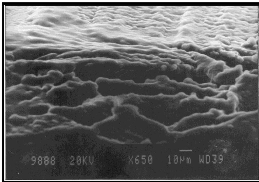
**Fig. 3: SEM photomicrograph of C.S of asymmetric membrane capsule (650X magnification)**
