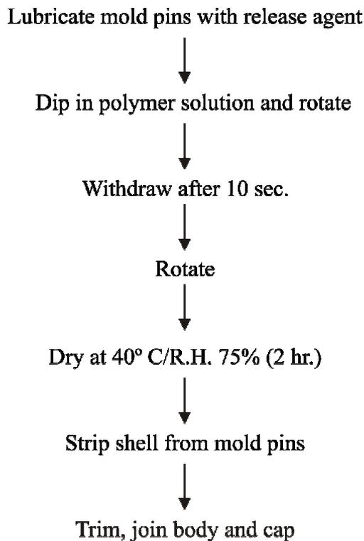
**Fig. 2: Manufacture of asymmetric membrane capsules by dry process method**
