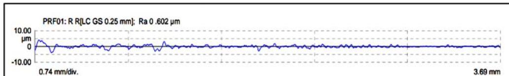
From the above graph reading the surface finish for milling No 9 is seem to be good i.e. surface finishing with 40% lubricant with three parameter speed of cut 6000 rpm, Depth of cut 0.8 mm, feed rate of 700 mm have the better surface finishing of  $R_a = 0.602 \mu\text{m}$ .
