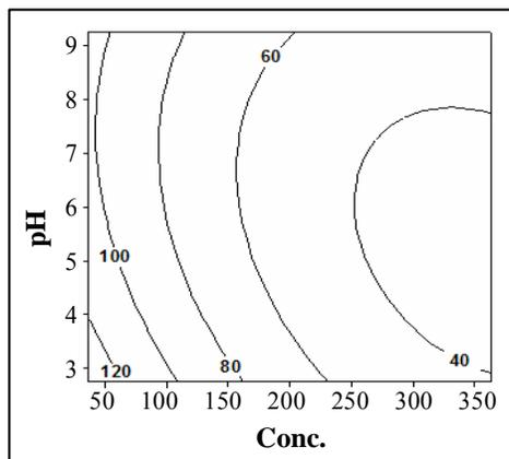
**Fig. 6 (c):** Response contour plot of % decolourization, pH and initial dye concentration
