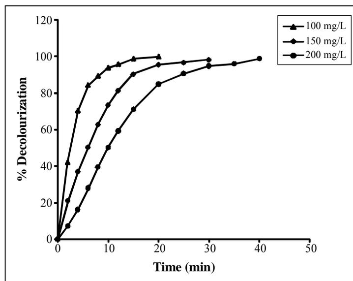
**Fig. 1: Effect of dye concentration on % decolourization (Conditions: pH: 6, H<sub>2</sub>O<sub>2</sub> concentration: 50 mM)**
