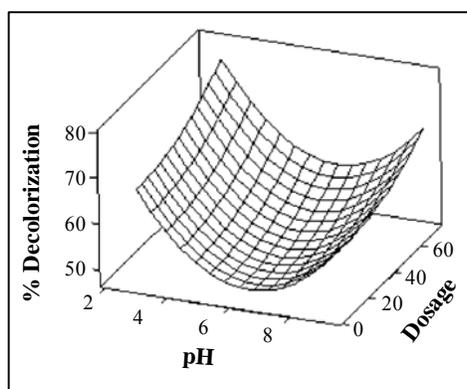
**Fig. 5 (c):** Response surface plot of % decolourization, pH and H<sub>2</sub>O<sub>2</sub> dosage
