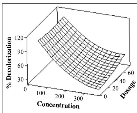
**Fig. 5 (a):** Response surface plot of % decolourization, initial concentration and H<sub>2</sub>O<sub>2</sub> dosage
