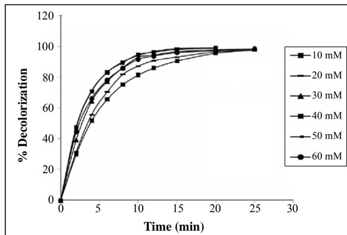
**Fig. 3: Effect of H<sub>2</sub>O<sub>2</sub> dosage on % decolorization (Conditions: pH 6, initial dye concentration 100 mg/L)**
