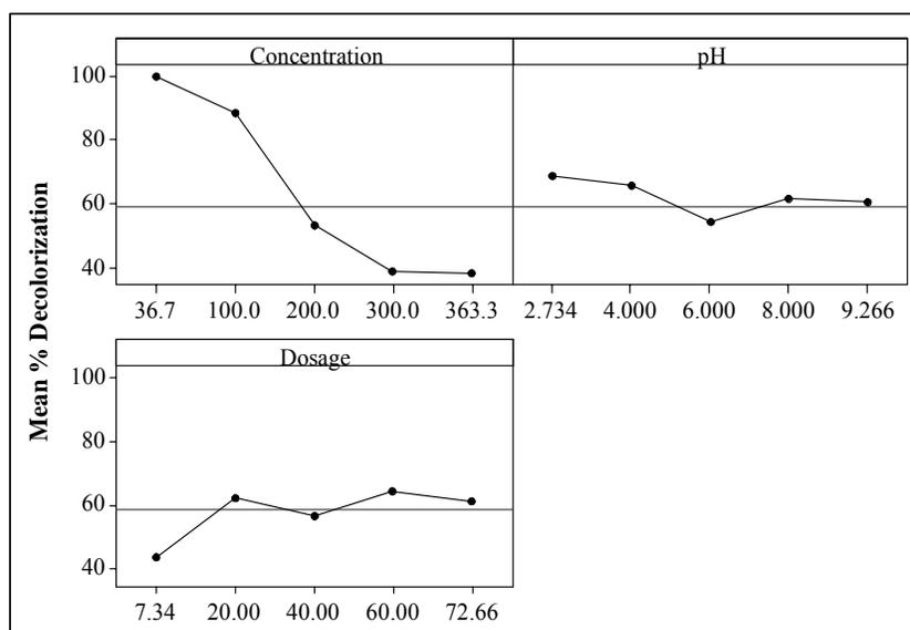
**Fig. 4: Main effects plot for % decolourization**
