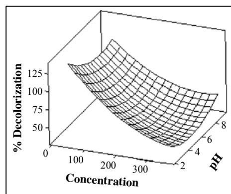
**Fig. 5 (b):** Response surface plot of % decolourization, pH and initial dye concentration
