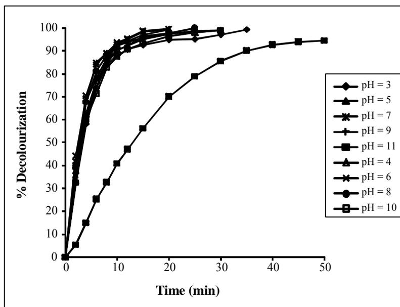
**Fig. 2: Effect of pH on % Decolourization**
