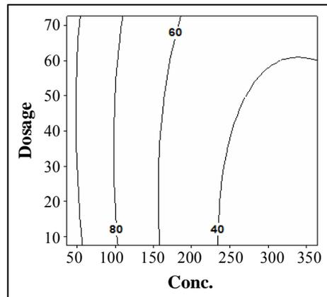
**Fig. 6 (b):** Response contour plot of % decolourization, initial dye concentration, H<sub>2</sub>O<sub>2</sub> dosage
