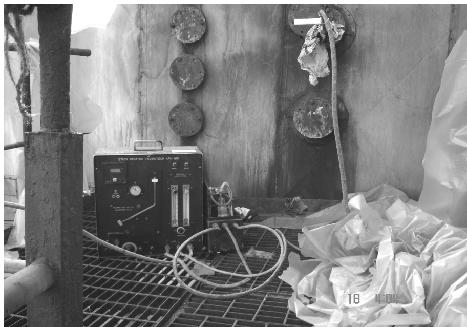
Fig. 1: Experimental set up using SO 2 monitoring kit for absorption of SO 2
