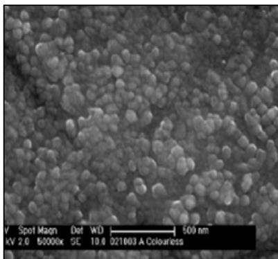
**Fig. 2: SEM Image of FeTiO<sub>2</sub> nanoparticles**
