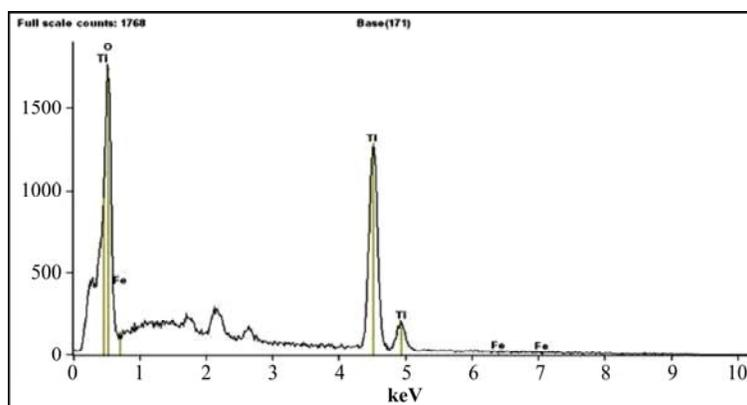
**Fig. 1: EDX analysis of FeTiO<sub>2</sub> nanoparticles**
