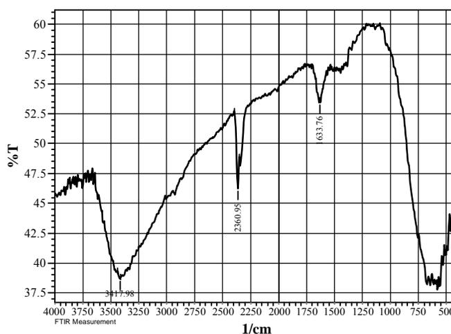
**Fig. 3: FT-IR Spectra of FeTiO<sub>2</sub> nanoparticles**
