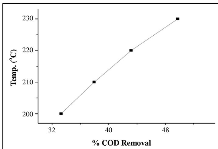
**Fig. 2: Effect of temperature on COD removal**
