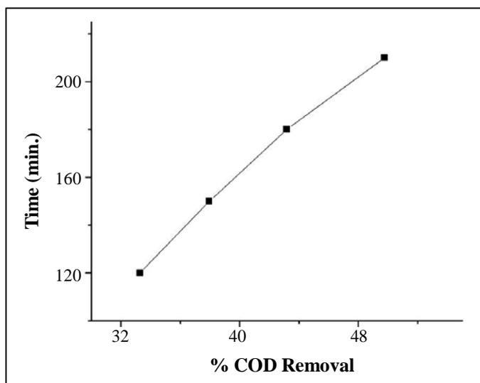
**Fig. 4: Effect of reaction time on COD removal**
