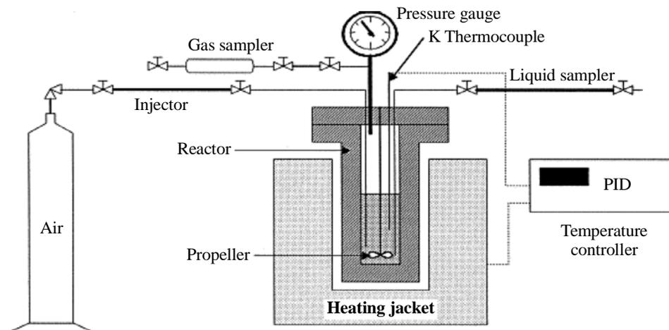
**Fig. 1: Thermal liquid-phase oxidation process unit (Basic flow diagram)**
