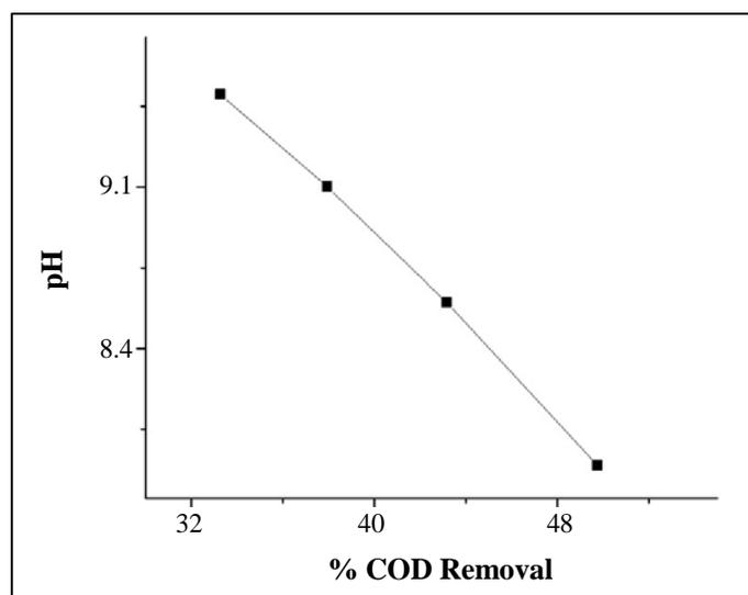
**Fig. 5: Effect of pH on COD removal**
