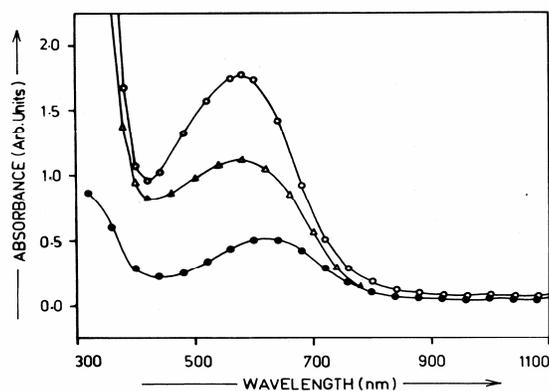
**Fig. 1: The optical absorption spectrum recorded for the (a) polyaniline (b) poly (o-methoxyaniline) and (c) poly (2,5-dimethoxyaniline) powder in DMSO solution**
