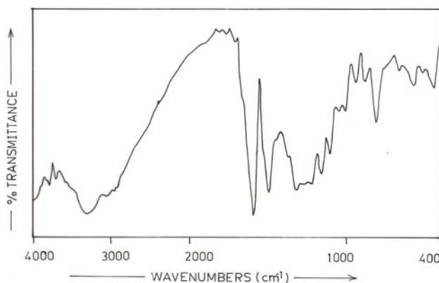
**Fig. 4: FTIR spectra of the chemically synthesized of poly (o-methylaniline) powder**
