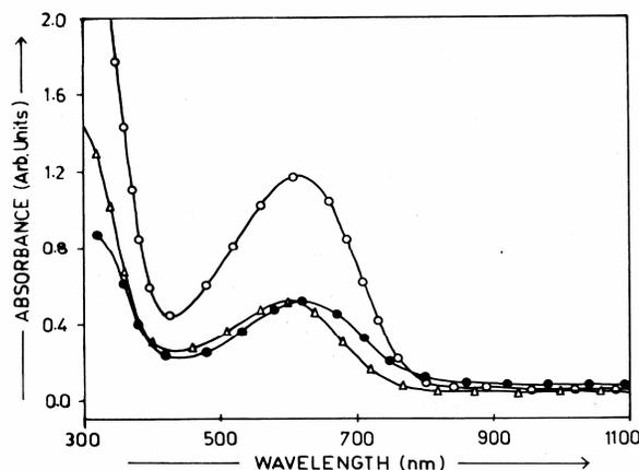
**Fig. 2: The optical absorption spectrum recorded for the (a) polyaniline (b) poly (o-methylaniline) and (c) poly(2,5 dimethylaniline) powder in DMSO solution**
