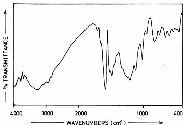
**Fig. 3: FTIR spectra of the chemically synthesized of poly (o-methoxyaniline) powder from oxalic**
