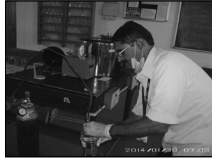
Fig. 9: Calorific value determination by Bomb calorimeter
