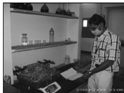
Fig. 7: Weighing of segregated MSW
