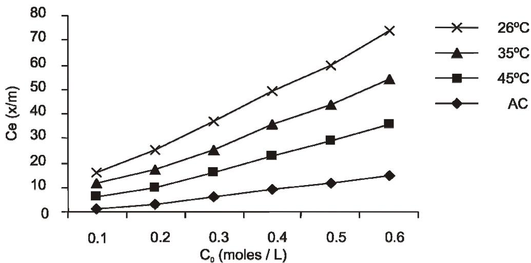
Fig. 2: Adsorption isotherm for oxalic acid on AC,  $C_{Zn}$  and  $C_{pH}$
