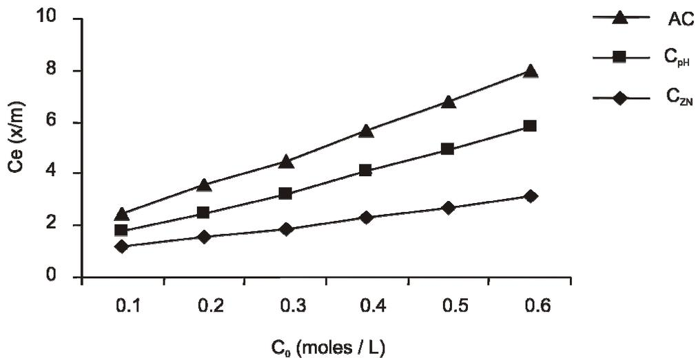
Fig. 1: Adsorption isotherm for oxalic acid on AC,  $C_{Zn}$  and  $C_{pH}$
