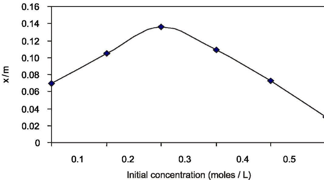
Fig. 3: Adsorption isotherm for oxalic acid on AC, CZn and CpH
