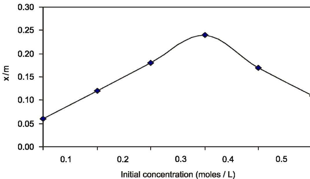
Fig. 4: Adsorption isotherm for oxalic acid on AC, CZn and CpH
