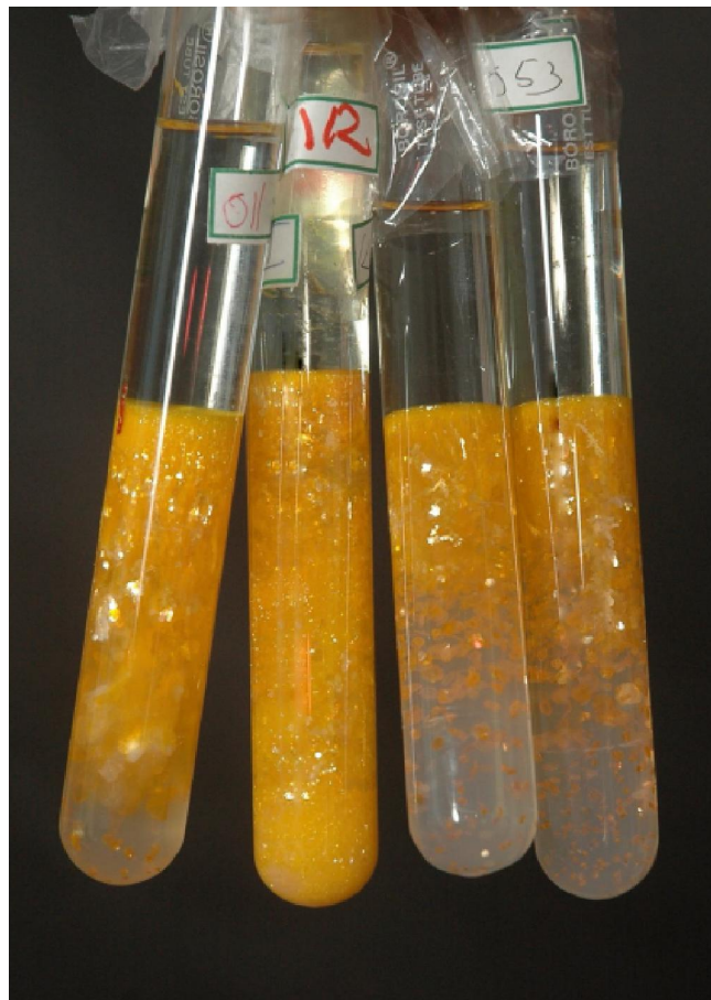
Figure 1 : Synthesis of lead iodide crystals in pure, electrifield, magneticfield, ultraviolet and infrared radiation grown samples
