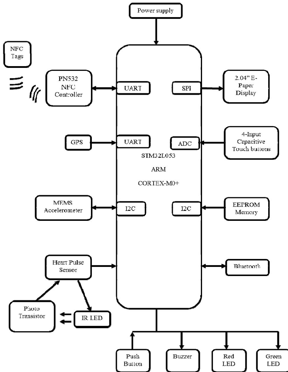
Fig. 1: Block diagram of wearable wrist band device
