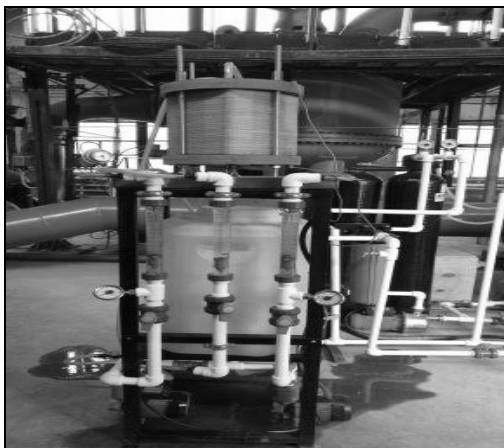
Fig. 1: A constructed electro dialysis unit
