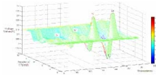
(b) Rectangular slot defects in the heat affected zone
