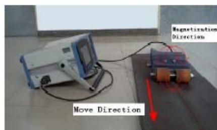
Figure 3 : Continuous non-contact scanning MFL system for the weld
