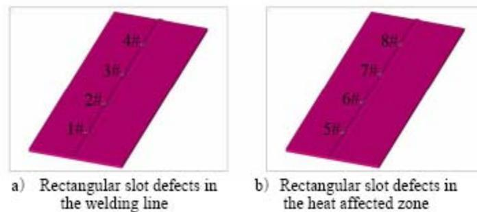
Figure 2 : Steel plate for testing
