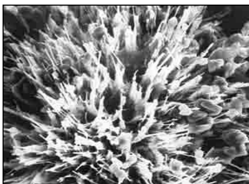
Porous structure of the concrete
