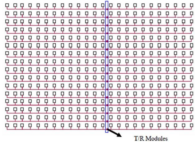
**Figure 1 : Planar array antenna of 24x16 radiating elements with 16 T/R module fed at each row**
