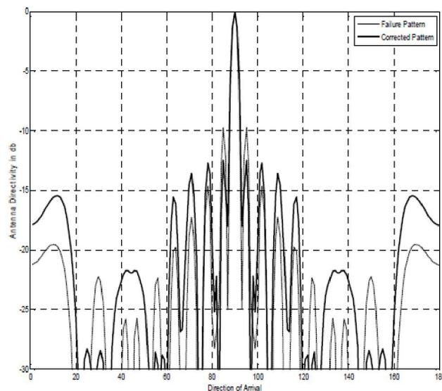
Figure 7 : Corrected pattern when elements of entire 12<sup>th</sup> and 13<sup>th</sup> row failures
