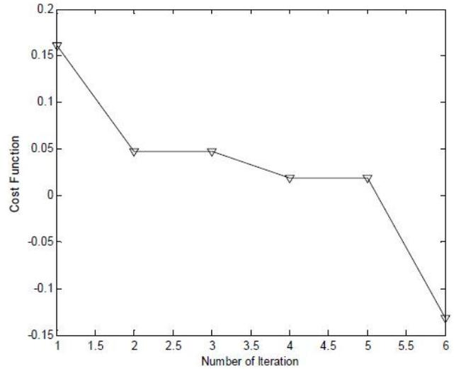
**Figure 4 : Fitness progress curves, obtained of 6 iterations, with main beam directed at broadside and elements of centre row failures**
