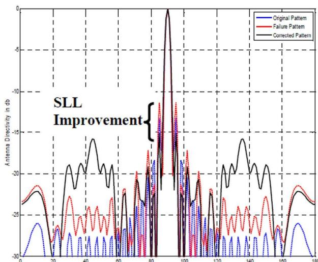
**Figure 3 : Corrected pattern with main beam pointing at broadside and failures at central row with original and uncorrected pattern**
