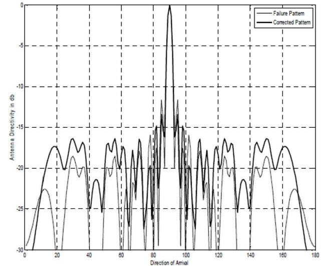
**Figure 5 : Corrected pattern when elements of entire 7<sup>th</sup> and 12<sup>th</sup> row failures with uncorrected pattern**
