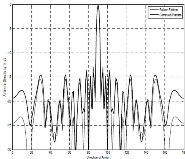
Figure 6 : Corrected pattern when elements of entire 7<sup>th</sup>, 2<sup>nd</sup> and 20<sup>th</sup> row failures
