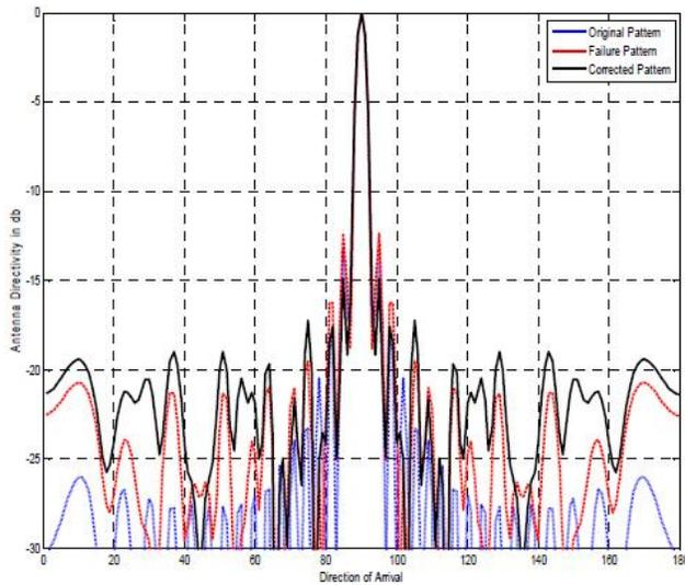
**Figure 2 : Corrected pattern along with original pattern and uncorrected pattern with main beam pointing at broadside considering the 9<sup>th</sup> row T/R module failure**
