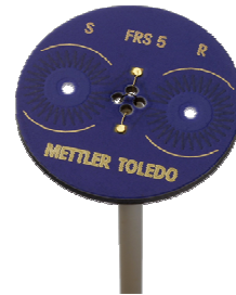
Fig. 2(b): Measurement principle of the FRS 5 interchangeable heat flux DSC sensor with 56 thermocouples 12
