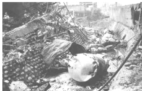
Fig. 1(b): Reactor bursts occurred by thermal runaway
