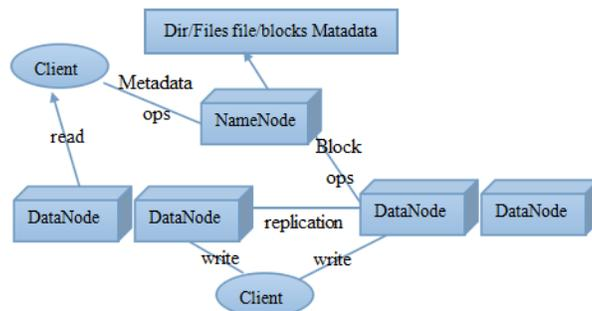
Figure 3 : The architecture of HDFS file system
