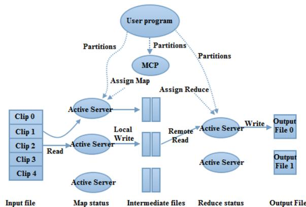
Figure 5: The operation execution process of Map Reduce
