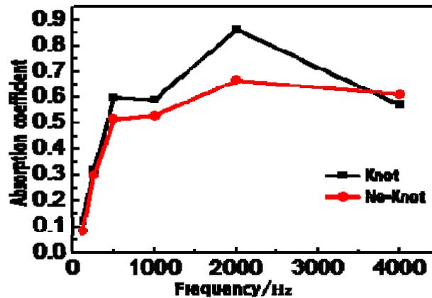
Figure 4 : The affection of knot on absorption characteristics
