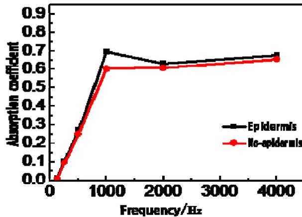
Figure 5 : The affection of epidermis on absorption characteristics
