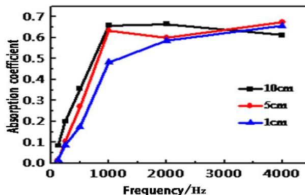
Figure 3 : The affection of sample thickness on absorption characteristics
