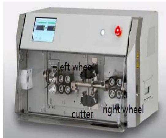
Figure 9: Stripping machine system working principle
