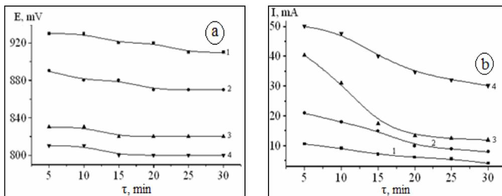
**Fig. 2:** Dependence of the EMF (a) и SCC (b) values from time in the galvanic pair of the system Fe-Fe<sub>2</sub>O<sub>3</sub> FeCl<sub>3</sub>, g/L: 1-10; 2-30; 3-50; 4-70
