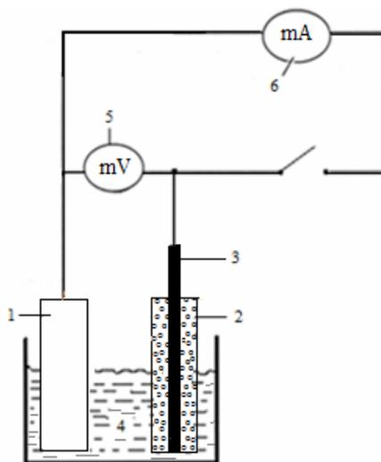
**Fig. 1: Installation for research of processes of formation of an electric current in system of galvanic pair Fe- $\text{Fe}_2\text{O}_3$**
