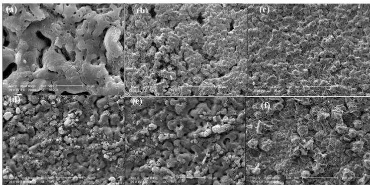
FIG. 1. SEM images from the surface of phosphate coatings in various amounts of nickel ion; a) 0 g/L b) 3 g/L c) 5 g/L d) 7 g/L e) 10 g/L f) 12 g/L.
