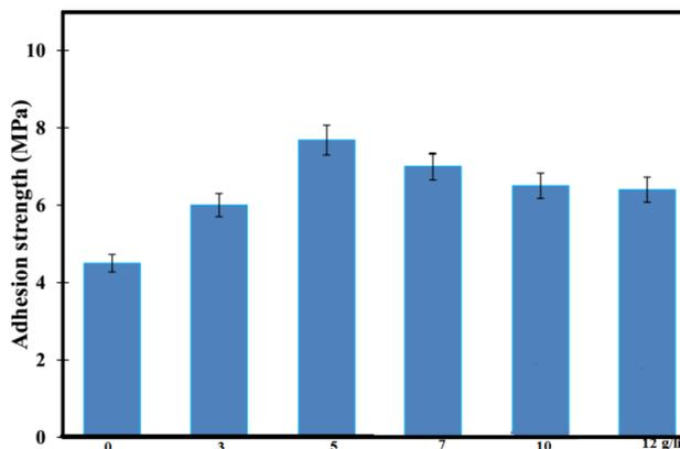
FIG. 2. Adhesion strength of epoxy coating applied on the phosphate coating with various amount of nickel ion.
