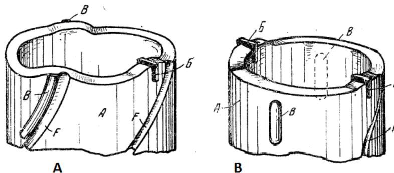
A-body; B-solid carbide cutters; C-Cemented carbide strips or islands; F-channels.
