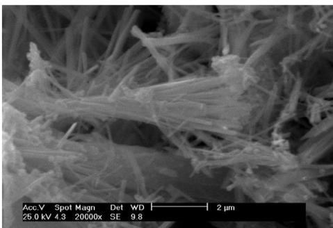
Figure 4 : SEM of  $\text{SrSnO}_2$  prepared at 400 °C
