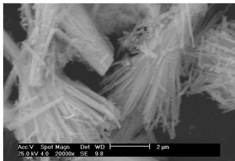
Figure 5 : SEM of  $\text{Sr}_2\text{SnO}_4$  prepared at 400 °C
