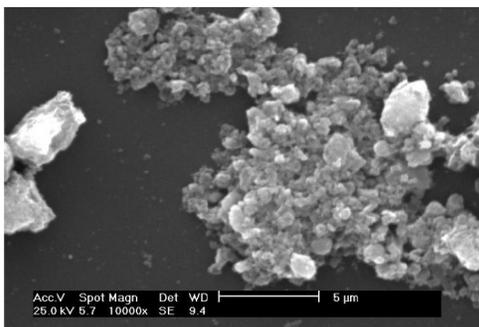
Figure 3 : SEM of  $\text{SnO}_2$  prepared at 400 °C
