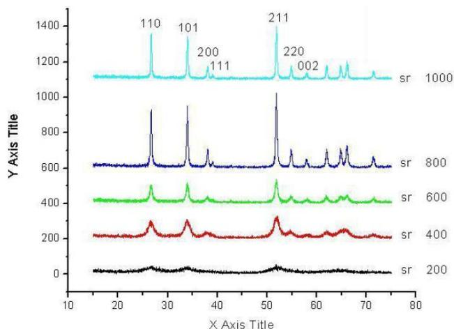
Figure 2 : X-ray diffraction patterns for nanoparticles  $\text{SnO}_2$
