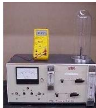
Figure 1 : Limiting oxygen index apparatus
