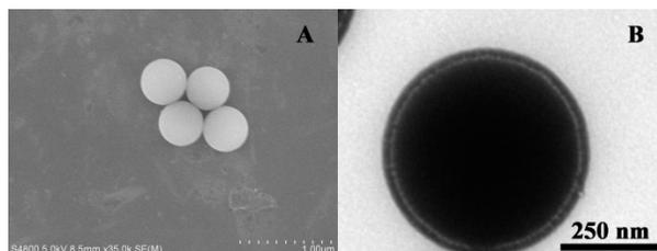
Figure 2 : SEM and TEM image of the *N*-halamine-grafted silica nanoparticles.
