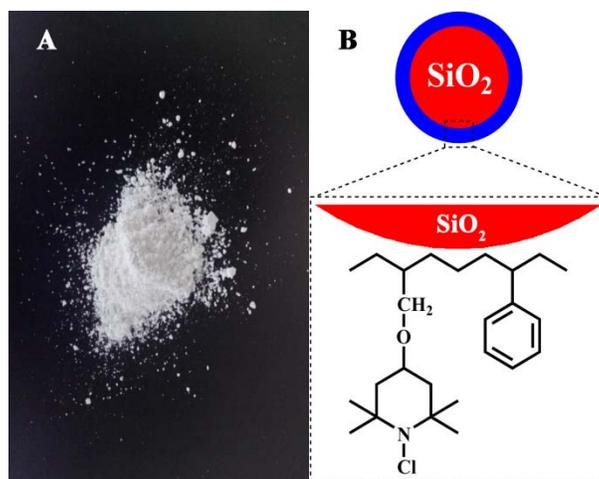
Figure 1 : The photo (A) and chemical structure (B) of the *N*-halamine-grafted silica nanoparticles.
