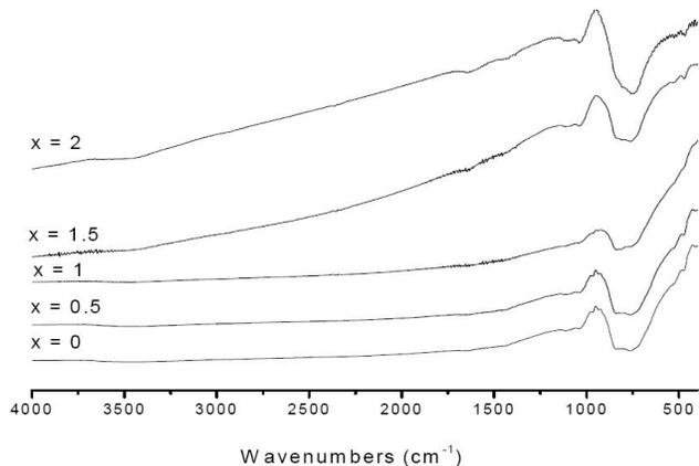
Figure 2 : Infrared spectra of  $\text{Pb}_8\text{Na}_{2-x}\text{Li}_x(\text{VO}_4)_6$  apatites.
