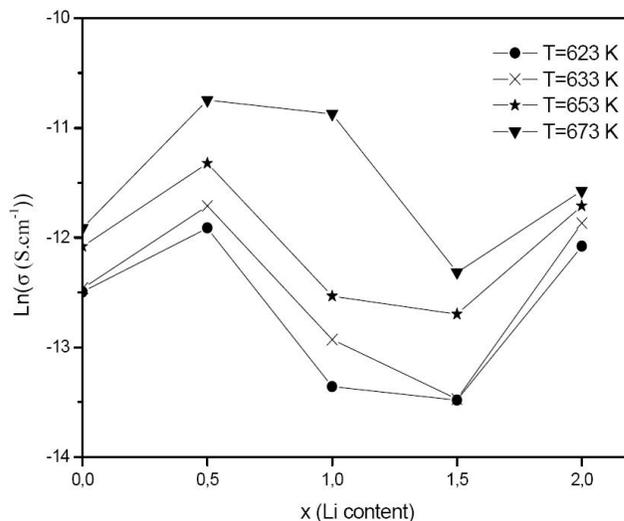
Figure 5 : Conductivity isotherms as a function of Li content (x) for  $Pb_8Na_{2-x}Li_x(VO_4)_6$  apatites.
