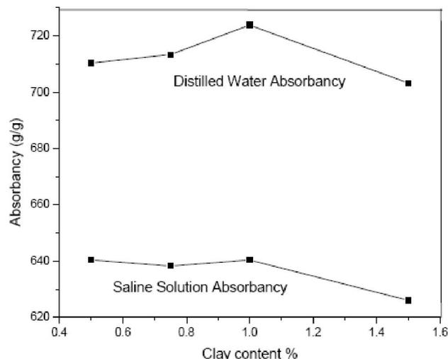
**Figure 7 : Effect of Clay Content on water absorbencies of the superabsorbent composites (Reaction conditions: Temperature: 70°C, 40 % degree of neutralization of AA, 1.25% Initiator and 1.25% Crosslinker, AA:Starch 3:1)**
