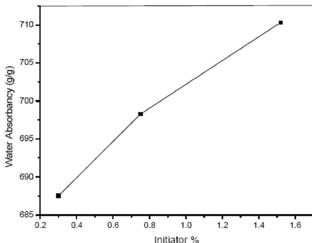
**Figure 5 : Effect of initiator content on distilled water absorbency of the superabsorbent**
