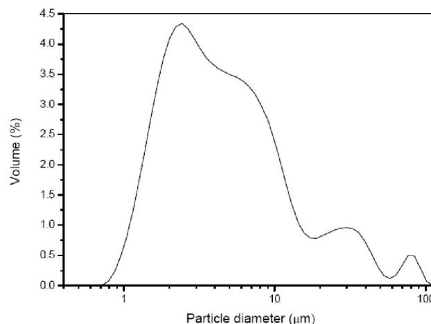
Figure 1 : Particle size distribution curve for Bentonite clay
