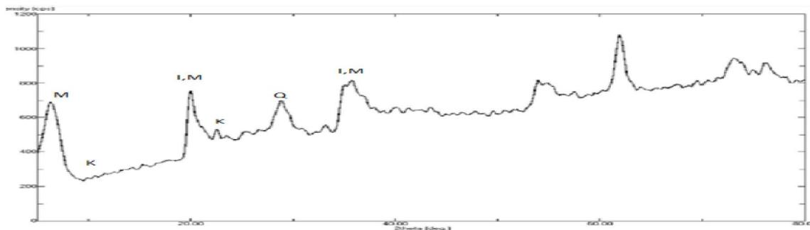
Figure 2 : X-ray diffraction pattern of Bentonite clay
