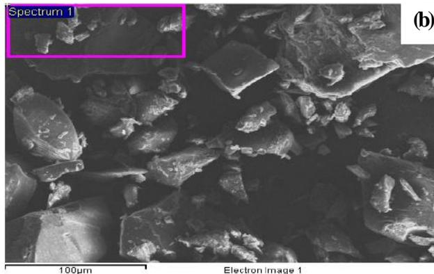
Figure 4 : Scanning electron micrograph of (a) crosslinked PAA & (b) PAA superabsorbent composite
