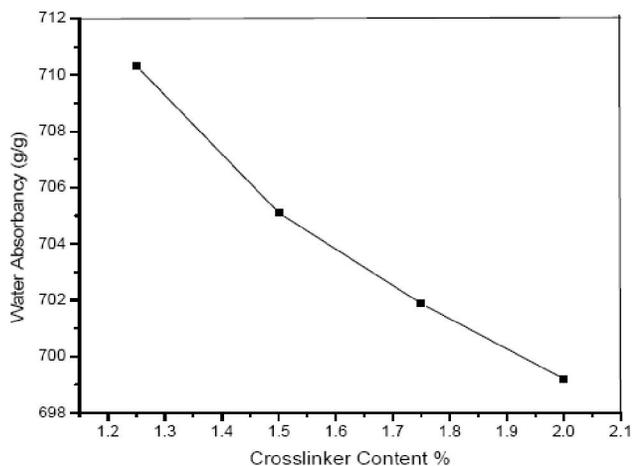
**Figure 6 : Effect of crosslinker content on distilled water absorbency of the superabsorbent (Reaction conditions: Reaction Temperature, 70°C, 40 % neutralization degree of AA, 0.5% clay, 1.25% initiator, AA:Starch 3:1)**
