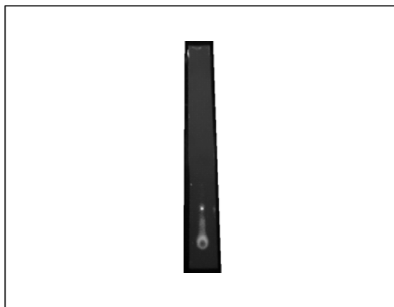
Fig. 1: TLC of second fraction of column of extraction of leaves and R_f value is 0.18 cm
